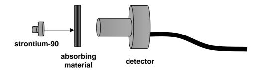
Different absorbing materials were placed between the strontium-90 and a radiation detector. The amount of radiation detected was noted for each absorbing material.
